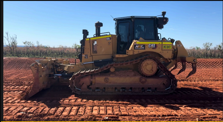
D6 VPAT LGP Dozers with Trimble Machine control
