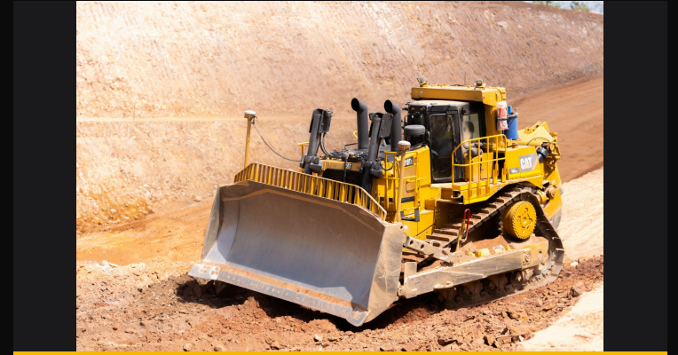
D10 Dozers with Trimble GPS
